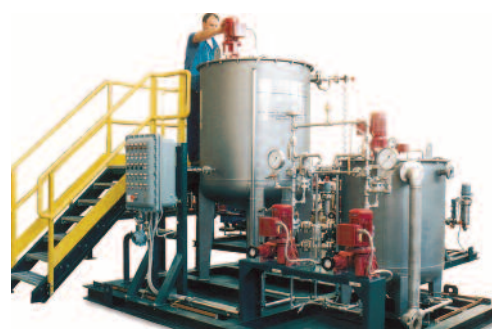
Phosphate Injection Package
