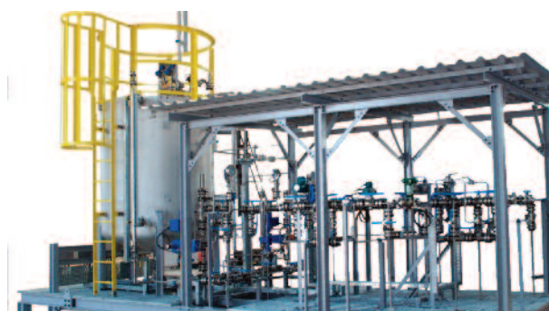
Chemical Injection Package
