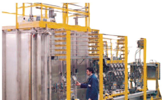
Corrosion inhibitor, Antifoam and Antiscale Injection Package
